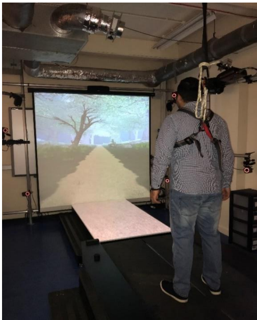
Figure 1 The CAREN System located at National Centre of Prosthetics and Orthotics, University of Strathclyde. The system is an advanced treadmill with integrated motion capture cameras. Furthermore, for safety the system has a harness that can hold the full body weight to prevent any falling.
