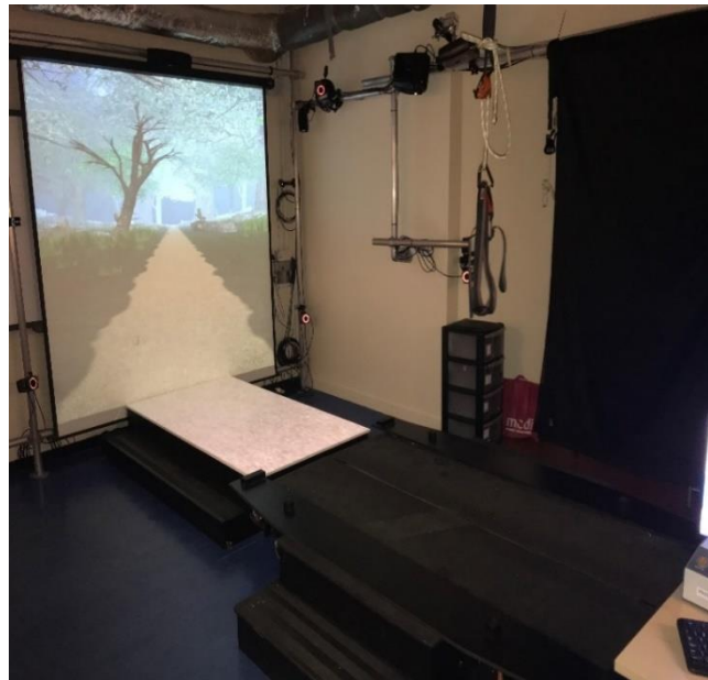
Figure 1 The CAREN System located at National Centre of Prosthetics and Orthotics, University of Strathclyde. The system is an advanced treadmill with integrated motion capture cameras. Furthermore, for safety the system has a harness that can hold the full body weight to prevent any falling.
